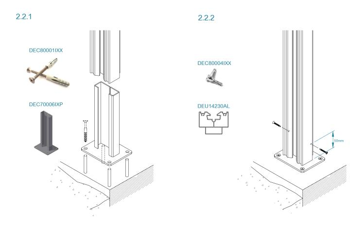
The installation surface should be completely flat and stable (e.g. 10 - 15 cm of solid concrete). .
