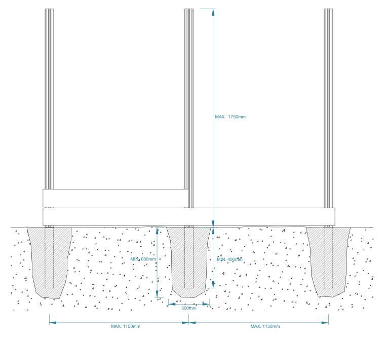
Open pits for foundation and secure the pillars with concrete
